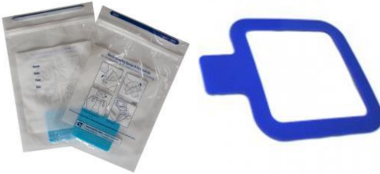
Figure 5.3 Sterile sponge, pre-soaked with saline solution (left) and sterile frame used for measuring the swabbed surface (right)
